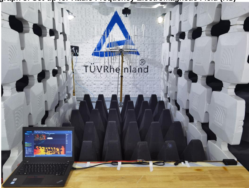
Photograph 3: Set-up for Radio Frequency Electromagnetic Field (RS)
